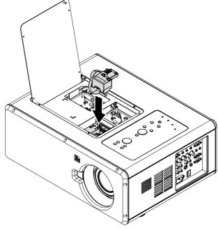
6. Close the lamp cover and secure the retaining screws as shown.
